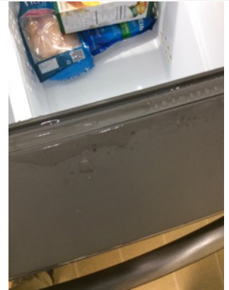
Water was seen on the freezer door.
