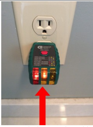
Reverse polarity was found in the electrical outlet in the half bathroom. Repair the outlet.
